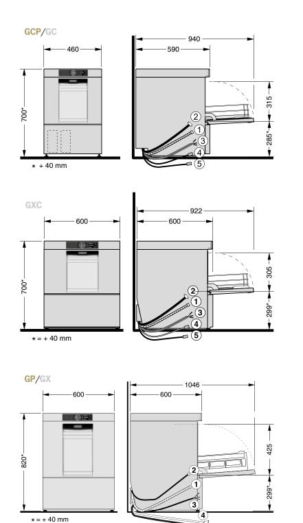
① flexible drain hose ② fresh-water connection ③ power cord
