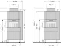
FTNi | FTPi-Dimensions Loading width: 612 mm and 760 mm Loading heigth: 440 mm
