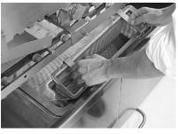
tanks. The basket opening is larger for easy cleaning and basket handles have been designed for easy lift-out access.
